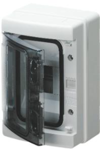
IP65 range of watertight enclosures from 4 to 72M with smoked transparent door. The main technical features are: reversible front and back panel, removable frames and panels with windows and detectable doors with up to 180° opening and lock accessory. The enclosures can be equipped with bipolar and unipolar terminal blocks, 80 A and 125 A, with screw wiring; they allow to create simple and neat wiring reducing the set-up time of the enclosure.
